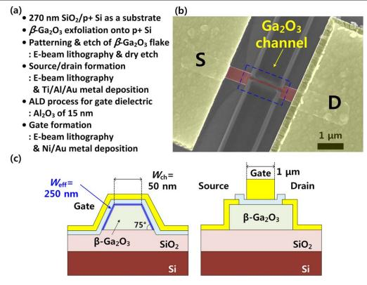
**Figure 1.** (a) Process flow for device fabrication of exfoliated tri-gate  $\beta$ -Ga<sub>2</sub>O<sub>3</sub> nano-membrane FETs with the top-gate structure. (b) SEM image of a fabricated device. (c) Cross-sectional schematics along both channel width and length directions.
