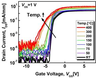
**Figure 3.** Measured  $I_{\rm DS}-V_{\rm GS}$  characteristics of the fabricated tri-gate  $\beta$ -Ga<sub>2</sub>O<sub>3</sub> FETs on SiO<sub>2</sub>/Si substrate at various temperatures ranging from RT to 400 °C.
