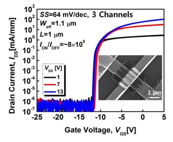
**Figure 5.** Measured  $I_{\text{DS}}-V_{\text{GS}}$  characteristics of the fabricated  $\beta$ -Ga<sub>2</sub>O<sub>3</sub> FETs with multi channels. Inset shows SEM image for top view of the fabricated device with 3 channels.
