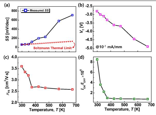
**Figure 4.** Temperature dependences (RT-400 °C) at  $V_{\text{DS}} = 1$  V of typical device parameters such as (a) SS (dashed line: Boltzmann thermal limit of SS), (b)  $V_{\text{T}}$ , (c)  $\mu_{\text{FE}}$ , and (d)  $I_{\text{ON}}/I_{\text{OFF}}$  of the tri-gate  $\beta$ -Ga<sub>2</sub>O<sub>3</sub> FETs on the SiO<sub>2</sub>/Si substrate.
