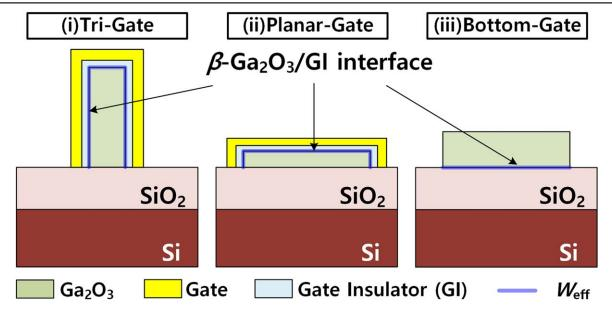
Figure 6. Schematics of cross-sectional view for the fabricated devices with different gate structures: (i) tri-gate, (ii) planar-gate, (iii) bottom-gate.
